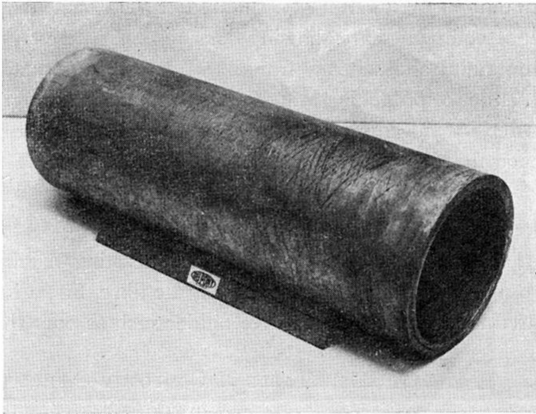
FIGURE 5. Filament wound Fibre FP/Al hollow cylinder. Fibre FP orientation: \pm 70^\circ/0^\circ/\pm 70^\circ/0^\circ/\pm 70^\circ .
